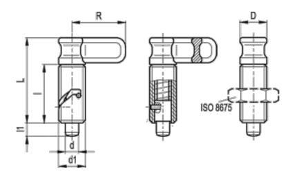
$\begin{array}{lll} D & = 16 \\ d - 0.02 - 0.04 & = 6 \\ d1 & = M16x1.5 \\ I1 & = 8 \\ L \ approx. & = 51 \\ I \ min & = 35 \\ R & = 32 \\ Spring \ pressure \ end \ (N) = 20 \end{array}$
